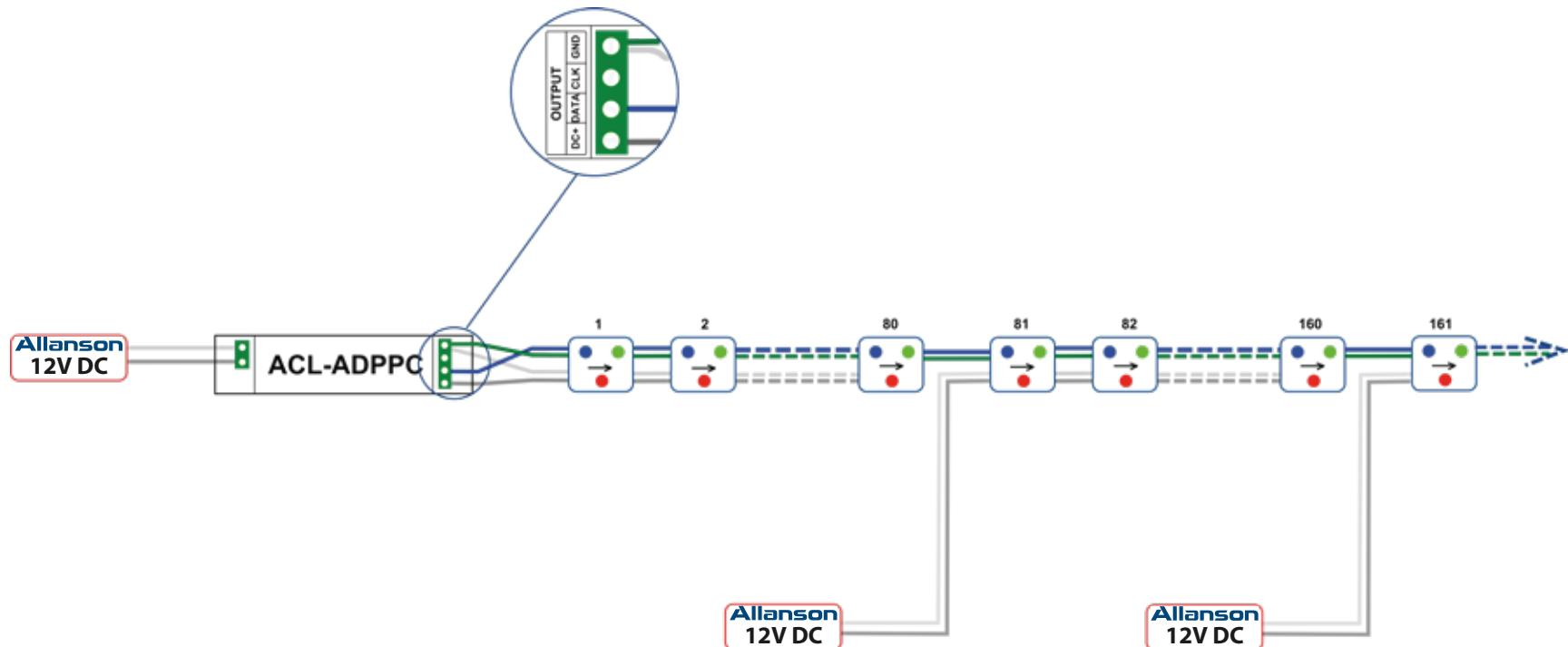
Each Allanson 60W Power Supply (CV125 series) can run maximum 80 modules.
