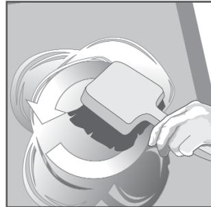
2. Concentrate on cleaning the image area using circular brush strokes.
