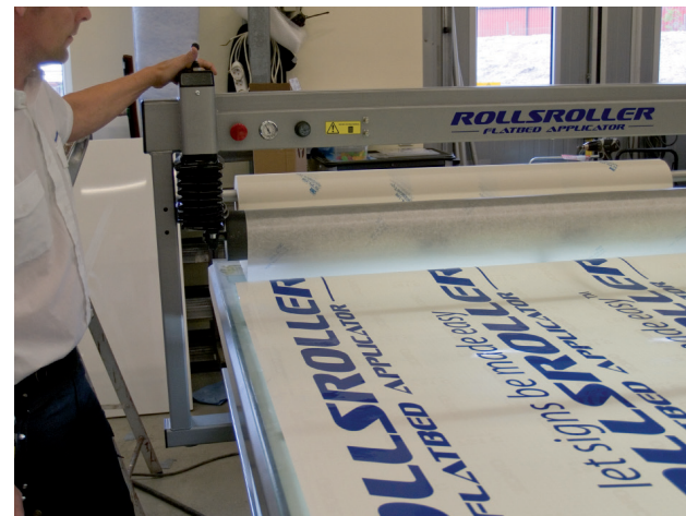
8. Raise the roller and pull it forwards slightly until the roller is positioned above the graphic. Make sure that the graphic is lying flat when you press the roller down. Now apply the tape over the graphic. Stop about 10 cm before reaching the end of the graphic.
