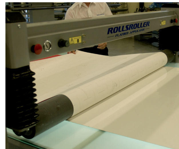
4. Fold half of the graphic film over the roller.
