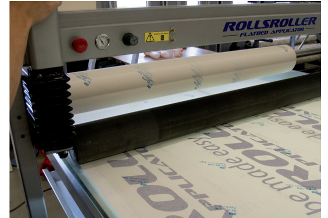
10. Push the glide beam back, press the roller down and apply the last piece of tape in the opposite direction.
