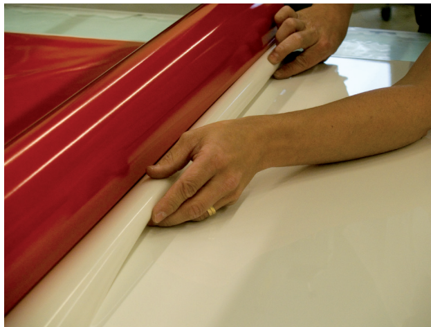
7. Fold the liner back underneath the roller ...
