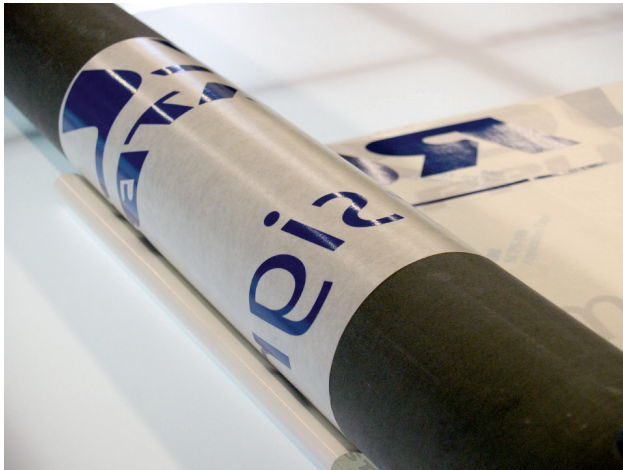
8. Apply half of the graphic using the roller. Press the roller down against the substrate.
