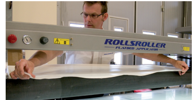
2. Pull out a length of application tape and fold it over the roller.
