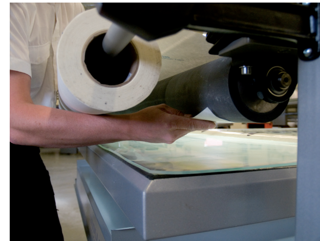
3. Take hold of the application tape underneath the roller ...
