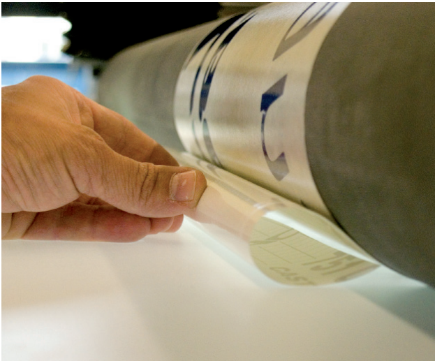
7. Fold the liner underneath the roller. Make sure it forms an even pleat.
