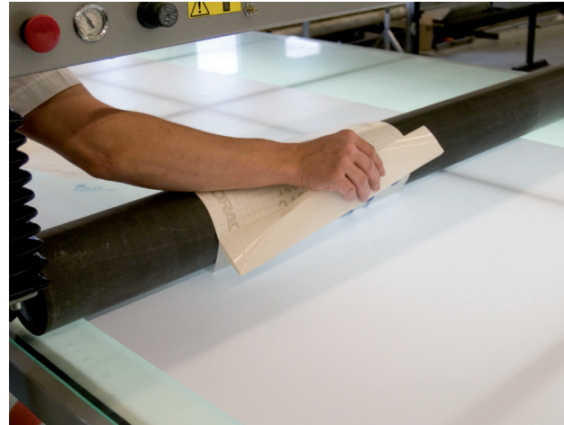
10. Take hold of the piece of liner you folded underneath the roller.
