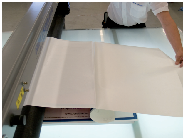
13. Apply the remaining part of the design to the substrate using the roller. Always remember to raise the roller slightly when it gets to the edge.
