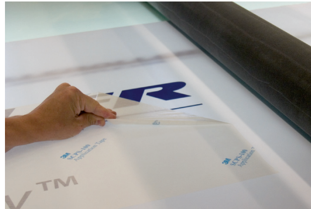
12. Remove the application tape, using the roller to hold the material in place.
