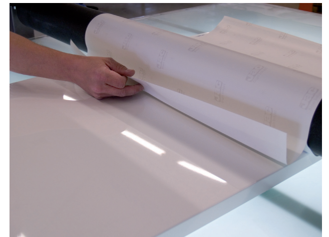
12. Take hold of the liner that you folded in from the other side. Move the glide beam over the surface. Always make sure that the graphic is pressed against the roller before starting application.
