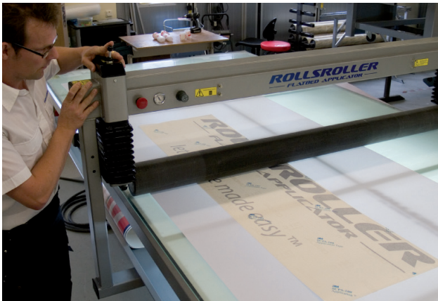
3. Press the roller down to fix the graphic into place.
