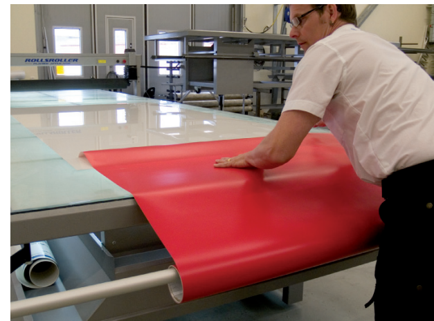
1. Place the sign material at the centre of the table and pull the graphic film over the substrate.
