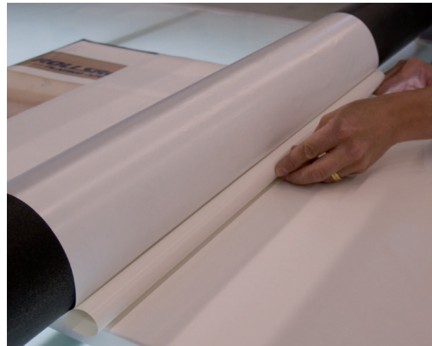
8. Fold the liner back underneath the roller to form an even pleat, as shown in picture.
