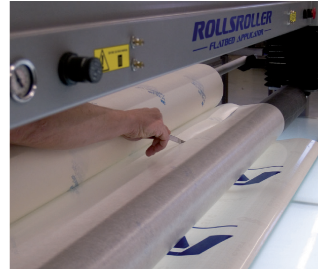
9. Trim before applying the last piece of tape. If you are applying tape to several graphics simultaneously, raise the roller and repeat the first steps in the same way as for the first graphics.
